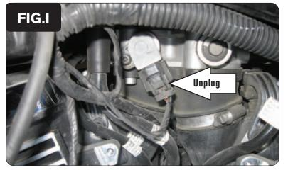
Locate the Throttle Position Sensor wiring harness on the left hand side of the throttle bodies. Unplug the stock wiring harness from the TPS (Fig. I).
