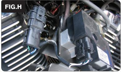
Plug the PCV wiring harness in-line of the stock wiring harness and Ignition Coil (Fig. H).
