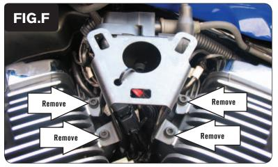
9 Remove the 4 bolts that hold the Ignition Coil bracket to the engine (Fig. F).
