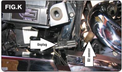
Locate the crank pickup coil connector on the right hand side of the bike near the rear shock (Fig. K).
