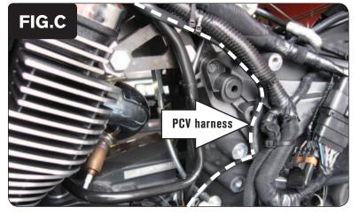
Route the PCV harness along the backbone of the frame along the left side of the bike and go towards the throttle body (Fig. C).
