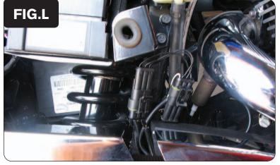
17 Plug the PCV harness in-line of the stock wiring harness and crank pickup coil connector (Fig. L).
