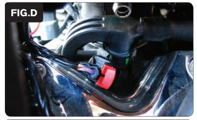
6 Locate the stock wiring harness at the rear injector (Fig. D). Lift the RED clip up and unplug the injector connector.
