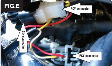
7 Plug the pair of leads with YELLOW colored wires from the PCV in-line of the stock wiring harness and the rear fuel injector (Fig. E)
