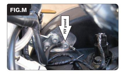
Attach the ground wire from the PCV to the stock ground location which is on the inside of the left engine case (Fig. M).
