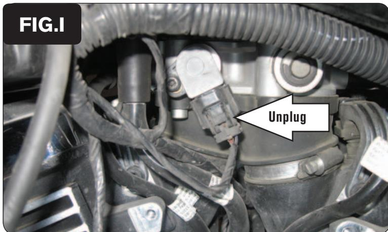
12 Locate the Throttle Position Sensor wiring harness on the left hand side of the throttle bodies. Unplug the stock wiring harness from the TPS (Fig. I).
