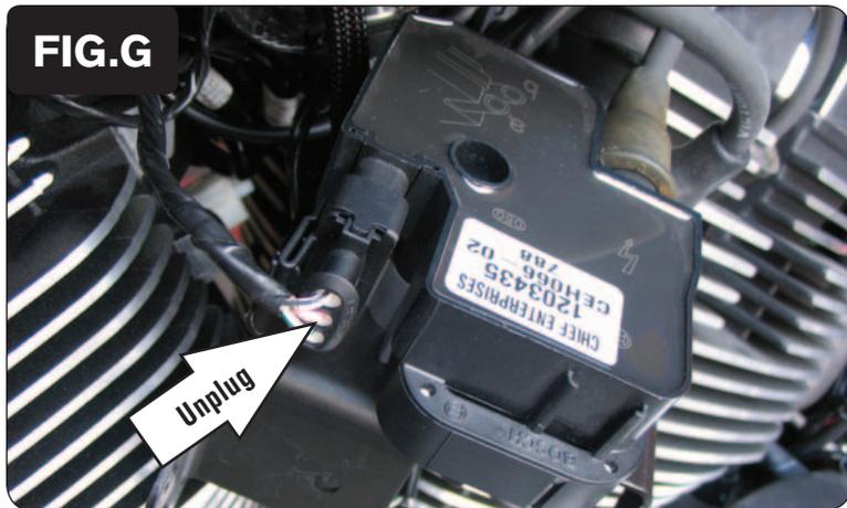
10 Unplug the stock wiring harness from the Ignition Coil (Fig. G).
